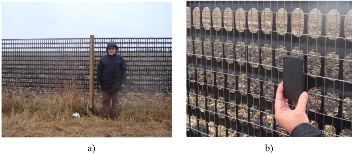
Figure 10.2: a) View of one of the lightweight plastic snow fences tested at the field site (A1 fence: P=50\% , G/H=0.34 , H \approx 1.9 ); b) Close view showing the 2 mm diameter welded wire frame used to support the plastic fence.
