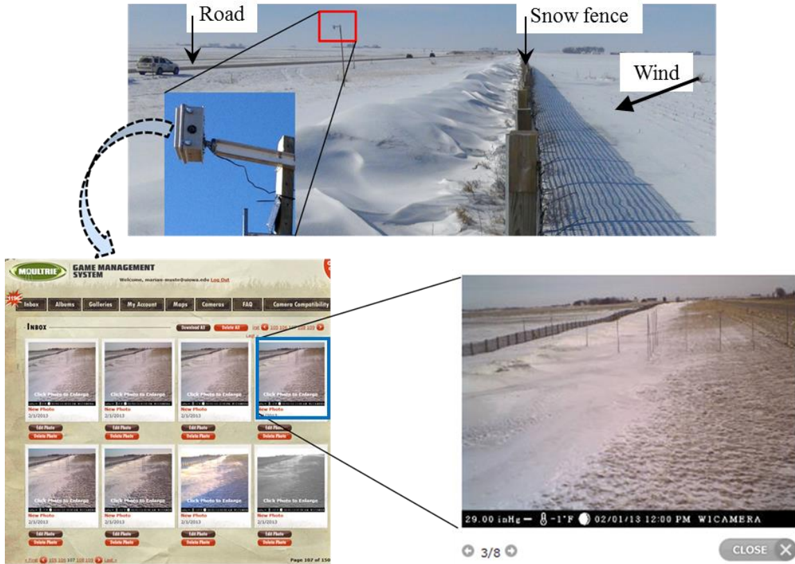
Figure 10.4 Field set-up and information provided by the real-time monitoring system.
